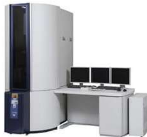
Gambar 16. Scanning Transmission Electron Microscope (STEM) Hitachi HD-2700 (Sumber: www.hitachi-hightech.com )
