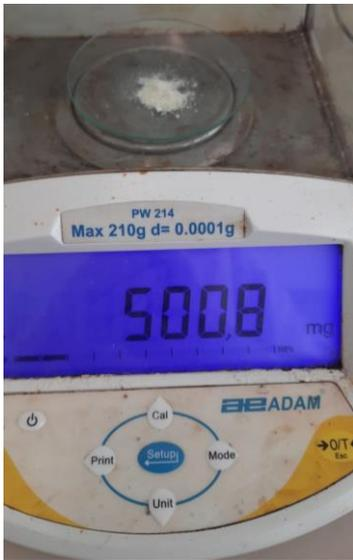
A digital scale (BEADAM PW 214) with a stainless steel weighing pan. The display shows 5008 mg. The scale has a power button, a print button, a setup button, a mode button, and a unit button. The maximum capacity is 210g and the readability is 0.0001g. |
