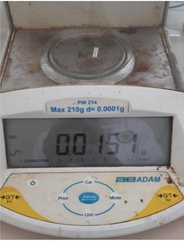
A digital scale (BEADAM PW 214) with a stainless steel weighing pan. The display shows a weight of 00.157 g. The scale has a maximum capacity of 210g and a readability of 0.0001g. The control panel includes a power button, a circular navigation pad with 'Cal', 'Print', 'Setup', 'Mode', and 'Unit' buttons, and two 'O/T' buttons.  |
