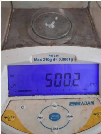
A digital scale (BEADAM PW 214) with a stainless steel weighing pan. The display shows 5002 mg. The scale has a power button, a print button, a setup button, a mode button, and a unit button. The maximum capacity is 210g and the readability is 0.0001g.  |
