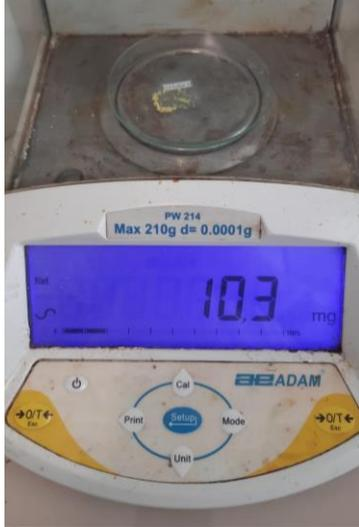
A digital scale (BEADAM PW 214) with a stainless steel weighing pan. The display shows 103 mg. The scale has a power button, a print button, a setup button, a mode button, and a unit button. The maximum capacity is 210g and the readability is 0.0001g. |
