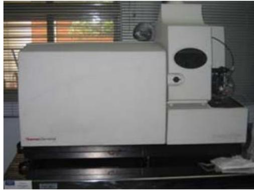
gambar 2 3. Instrument ICP-MS (Irzon, 2018).
