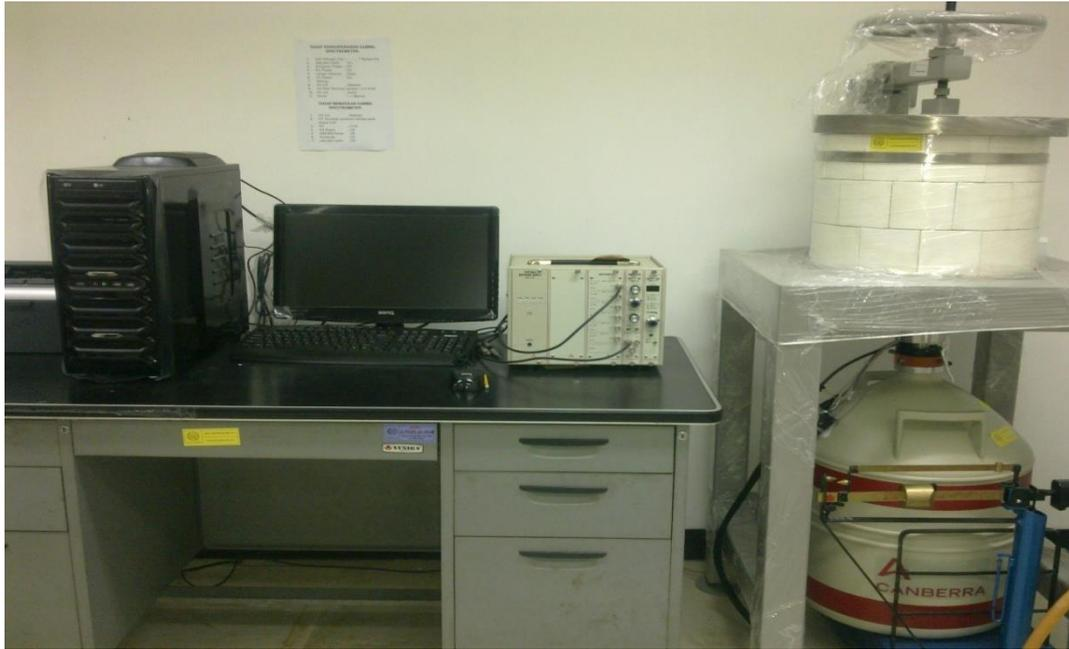
Gambar 5. Alat *Multi Channel Analyzer* (MCA) Spektrometer Gamma
