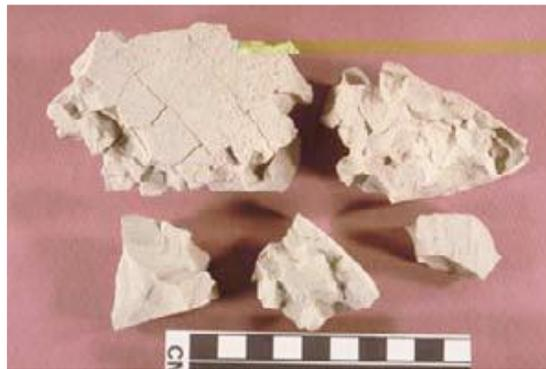
Gambar 3. *Montmorilonite* (Bentonit)
