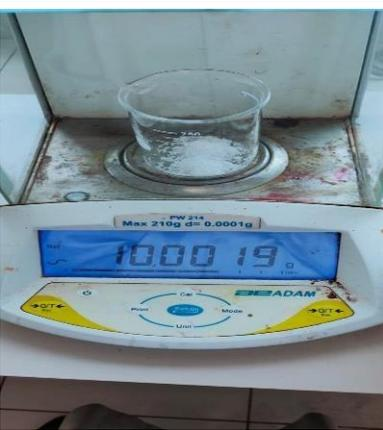
A photograph of the analytical scale with a glass beaker placed on the weighing pan. The display shows a reading of 10.0019 g. The beaker contains a white powder.                                                                      |
