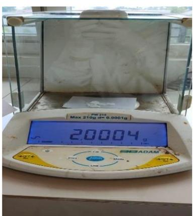
A photograph of the same analytical scale with the weighing chamber open. The display shows a reading of 2.0004 g. A small amount of white powder is visible on a piece of paper inside the chamber.                                     |
